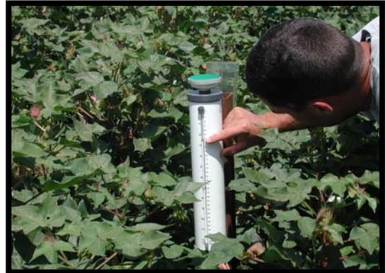
Fig. 1. Measuring potential ET in SDI management plots with an ET gauge.
