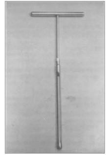
Figure 1: Soil Probe
