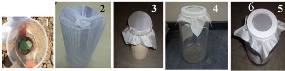
Figure 2. Cage types evaluated previously: 1) transparent plastic cup cage, 2) wire mesh sleeve cage, 3) opaque plastic cylinder, 4) transparent plastic jar without ventilation, and 5) transparent plastic jar with ventilation.
