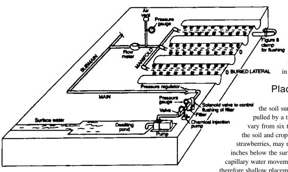
water leaves the tube. In a freshly installed system, the loose soil may settle around a collapsed tube, making it difficult for the tube to regain its shape in absence of an air vent. A typical field layout is shown in Figure 1.
