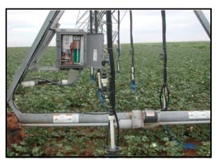
Figure 2. Remote terminal unit activating valves on Spans 7 and 8 of the VR irrigation system, TAES, Helms Farm. 2001
