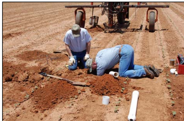
Installation of volumetric soil water sensors for comparison to neutron probe water measurement, Helms, 2007.
