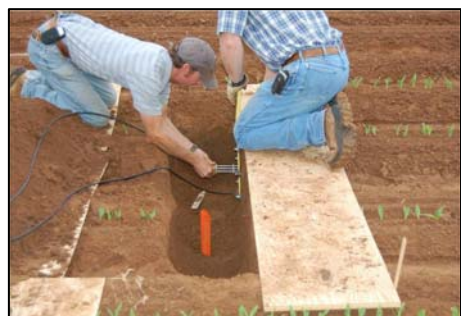
Fig. 1 Installation of TDR sensors for measuring volumetric soil water content in an array above and to each side of the drip lateral.
