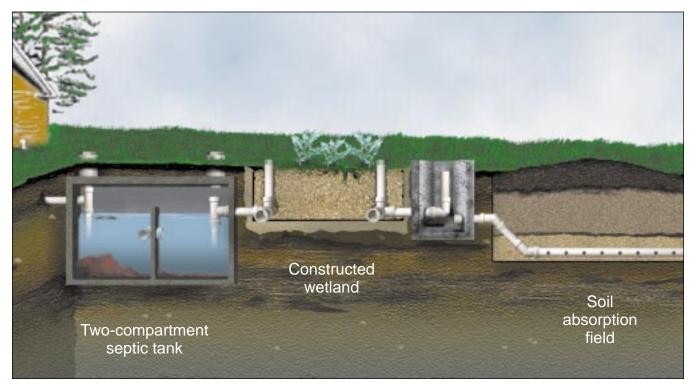
Figure 1: A constructed wetland system.
