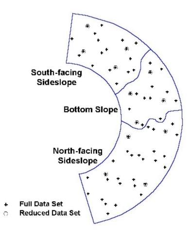
Fig. 2. Half-acre-grid soil sampling and six sub-samples per zone, Ropesville, Lamesa, TX
