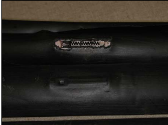
Fig. 1. SDI emitter and emitter flow path that is plugged by Mn precipitates coming from the irrigation water supply, Helms Farm, 2002..
