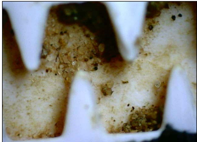
Fig. 2 Deposits of sand particles with no indications of MnO_2 precipitation in a magnified drip emitter pathway, TAES, Halfway, 2005.
