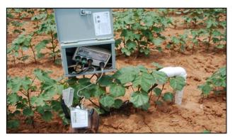
Fig. 1. Data logger and recorder for TDT soil sensors located in a drip irrigated cotton field at the Helms Research farm, 2007 and 2008.
