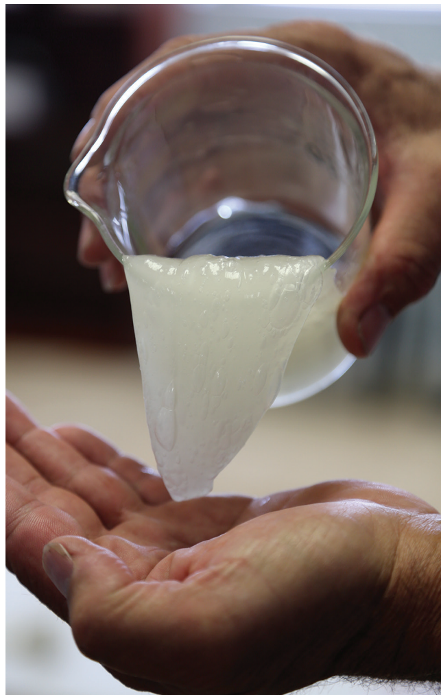
A borate crosslinked guar fluid system, illustrating its viscosity, is shown at PfP Technology.
