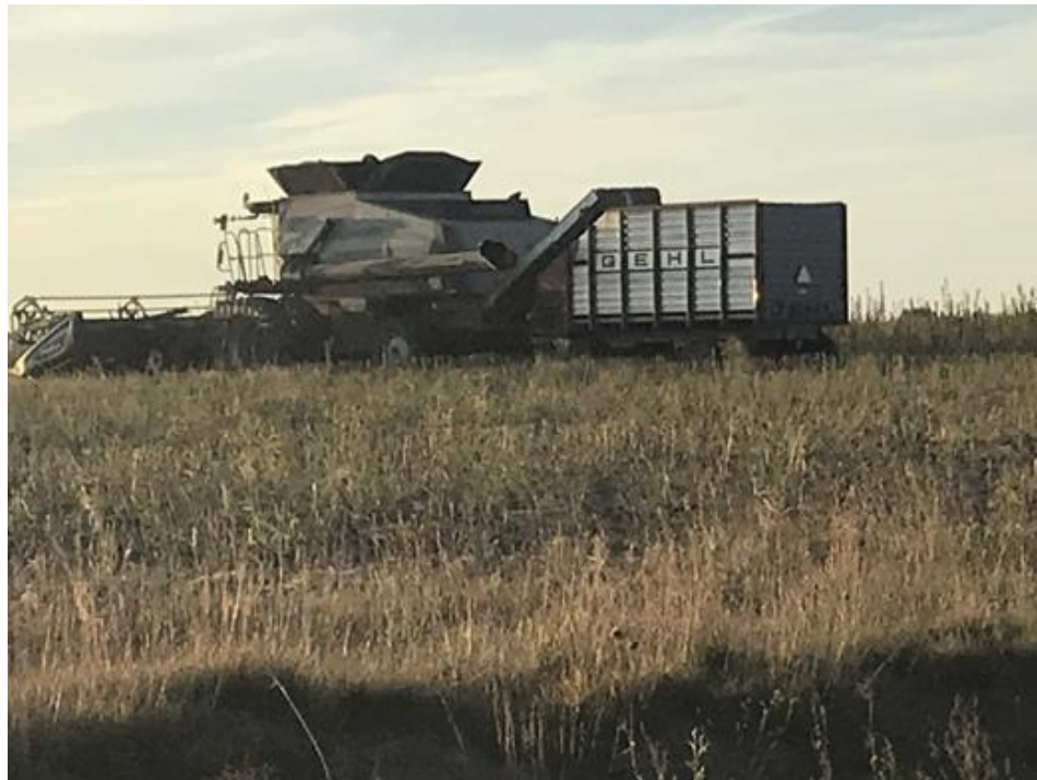
A modified Gleaner combine harvests hemp for floral structures and grain near Springfield, CO., in 2018. The combine cuts the top of the plant and separates the flower bracts (containing CBD) and the grain. Flower bracts are discharged into a towed GEHL buggy that then hauls to a baler/compactor that wraps the small round bales in plastic.
